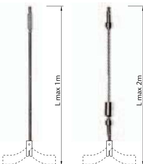
**N.B.** IL CONTROLLO DI LIVELLO VIENE FORNITO NELLA VERSIONE BASE COME DA FIGURA A SINISTRA (RL-A STANDARD). L'ESTENSIONE O PROLUNGA PUÒ ESSERE AD ASTA CON LUNGHEZZE STANDARD DA 500 E 1000 mm ACCORCIABILI OPPURE A FUNE CON LUNGHEZZA DI 2000 mm ACCORCIABILE. LE ESTENSIONI VANNO ORDINATE SEPARATAMENTE DALLA VERSIONE BASE DEL CONTROLLO DI LIVELLO E NON SONO COMPRESIVE DI ELICA.
